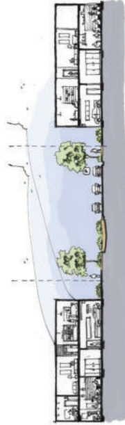
Figure 4.3.9 Local access street (16m) - typical section
